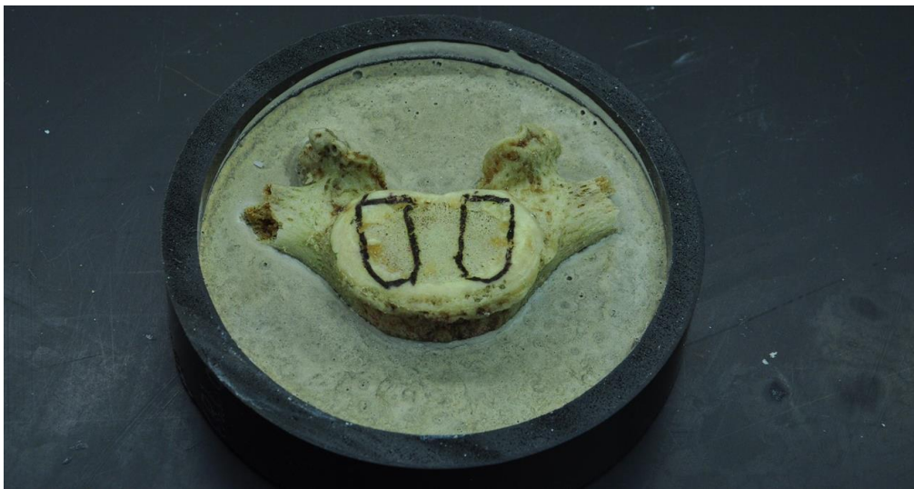
Figure 5. L5 vertebra potted in cement for biomechanical testing.
